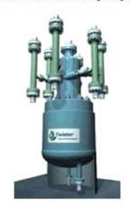
The LTX vessels are multi-phase low temperature separators which have been manufactured by KNM in Malacca under sub-contract from Twister BV. The vessels are clad in Inconel 625 and each one measures 3.5 metres in length and 1.7 metres in diameter, weighing 18,000 kgs. The vessels have been manufactured in accordance with a proprietary (patented) Twister BV design which efficiently separates gas, water and condensate whilst managing hydrate formation without the use of chemicals.
